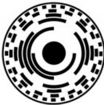
Absolute Encoder Disk (8-bit)
