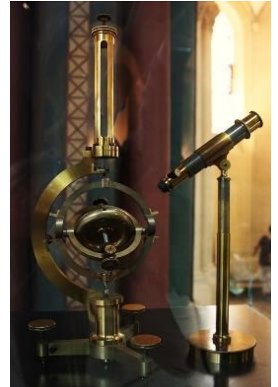
Gyroscope invented by Léon Foucault in 1852 (Replica)
