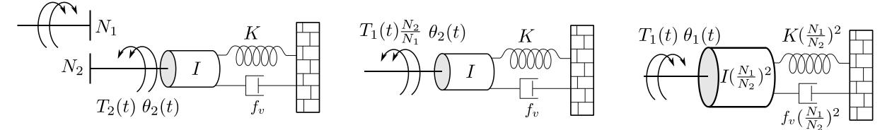
$$(Is^{2} + f_{v}s + K)\theta_{2}(s) = T_{1}(s)\frac{N_{2}}{N_{1}} \Rightarrow (Is^{2} + f_{v}s + K)\frac{N_{1}}{N_{2}}\theta_{1}(s) = T_{1}(s)\frac{N_{2}}{N_{1}}$$
